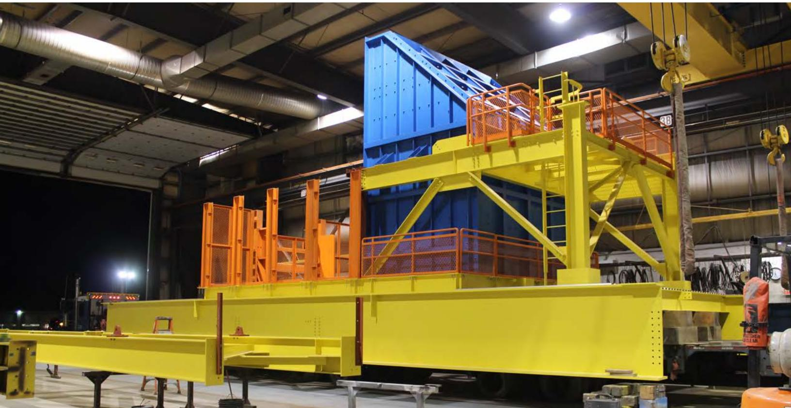
The completed modules for the Mosaic project were very large - up to 29 feet tall x 23 feet wide x 61 feet long - and weighing up to 90 tons. An important part in the project scope involved the test-fit of the modules off-site before delivery. This would confirm that all the fabricated components fit together as designed – and that the process could be repeated, with no fit-up issues on site during installation.
